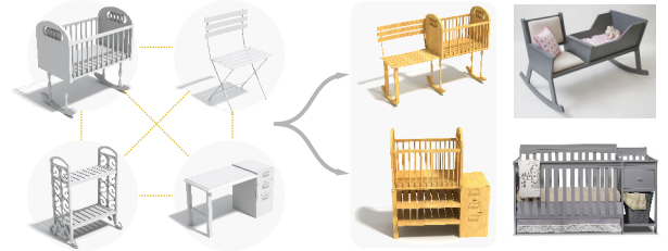
Fig. 1: Starting from a heterogeneous collection of four objects (left) as initial population, our functionality-aware evolution tool can generate a variety of plausible hybrid shapes. Two of them (middle) exhibit strong functional similarity to existing professional designs (right).
