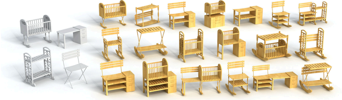
Figure 6.4: Starting from a heterogeneous collection of four shapes (in gray) as initial population, our functionality-aware modeling tool is able to generate a variety of offspring shapes (in yellow) with a combination of constrained and unconstrained evolution. Some of the offspring shapes exhibit forms of cross-category structure breaking.
