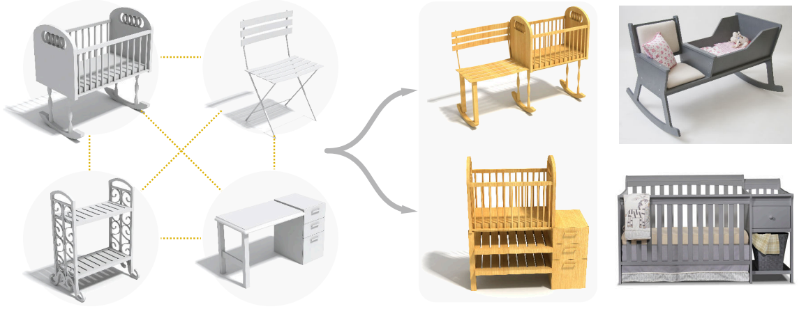
Figure 1.2: Starting from a heterogeneous collection of four objects (left) as initial population, our functionality-aware model evolution can generate a variety of plausible hybrid shapes. Two of them (middle) exhibit strong functional similarity to exiting professional designs (right).
