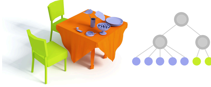
Figure 4.3: The ICON descriptor (right) that describes the interactions of the table in orange in the scene (left). Using the ICON descriptor, the interactions of the table are organized into a tree structure, where the leaf nodes (blue and green nodes) represent the interacting objects and the internal nodes (gray nodes) group the leaf nodes with similar interactions. The image is courtesy of Hu et al. [25].
